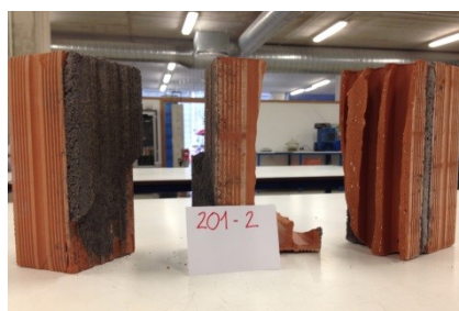
MSap 2 Shear stress breakage of the ceramic brick
