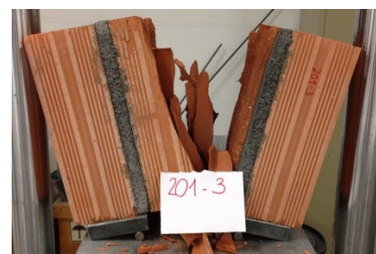
MSap 3 Shear stress breakage of the ceramic brick
