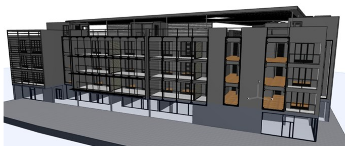
Fig. 4: Front elevation of virtual building created with the help of BIM software (source: own study)
