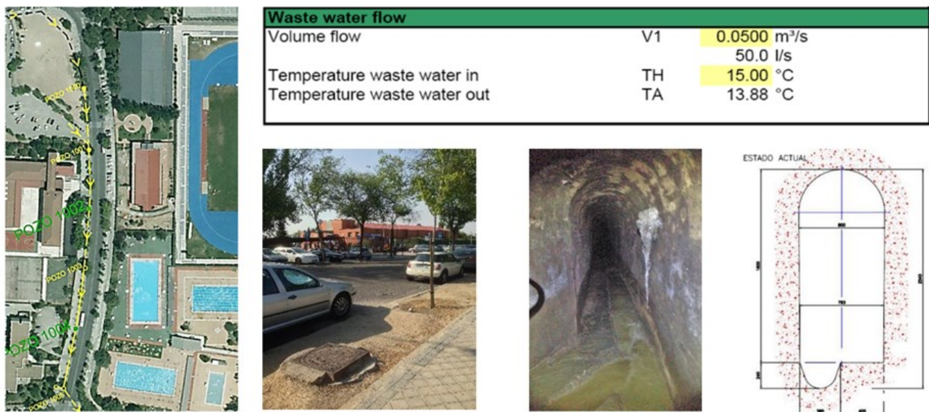
Figure 5: Very close to the CDM runs an accessible wastewater collector an average temperature of 15 °C and with an average flow of 50 L/s = 180 m 3 /h. A continuous and free resource of wasted energy and a huge efficiency opportunity.
