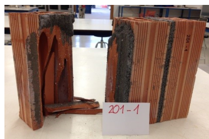
MSap 1 Shear stress breakage of the ceramic brick
