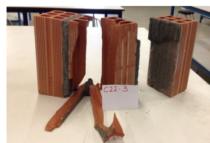
MSwr 3 Shear stress breakage of the ceramic brick
