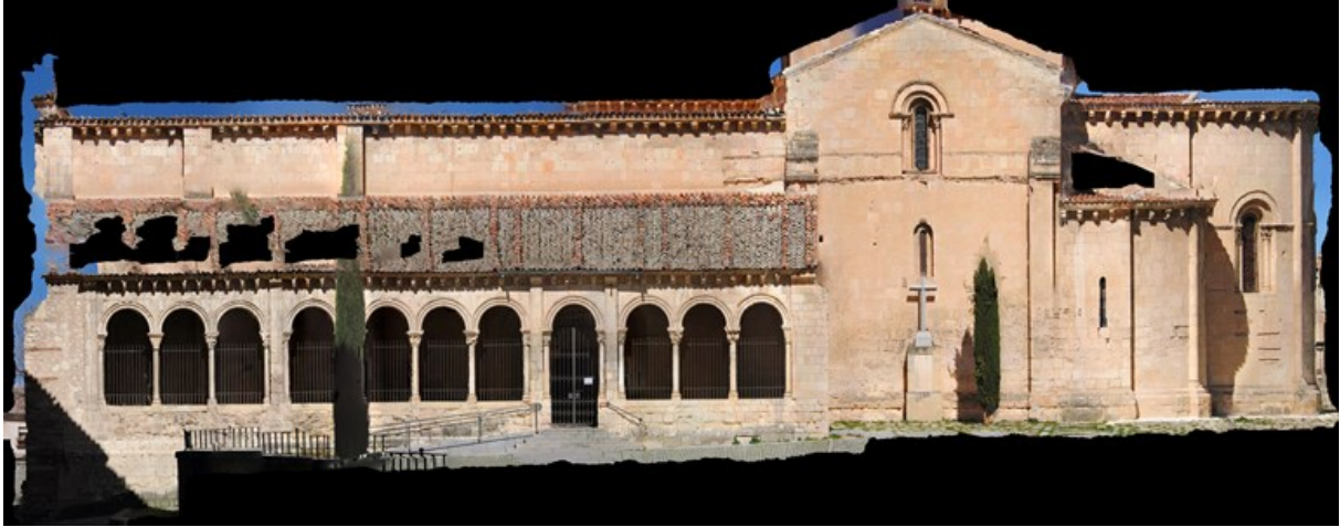
Figure 2. Orthophoto obtained with Agisoft PhotoScan Professional software and exported to JPEG.
