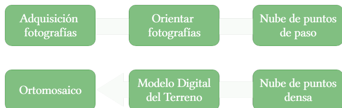
Fig. 3. Workflow used in photogrammetric software.
