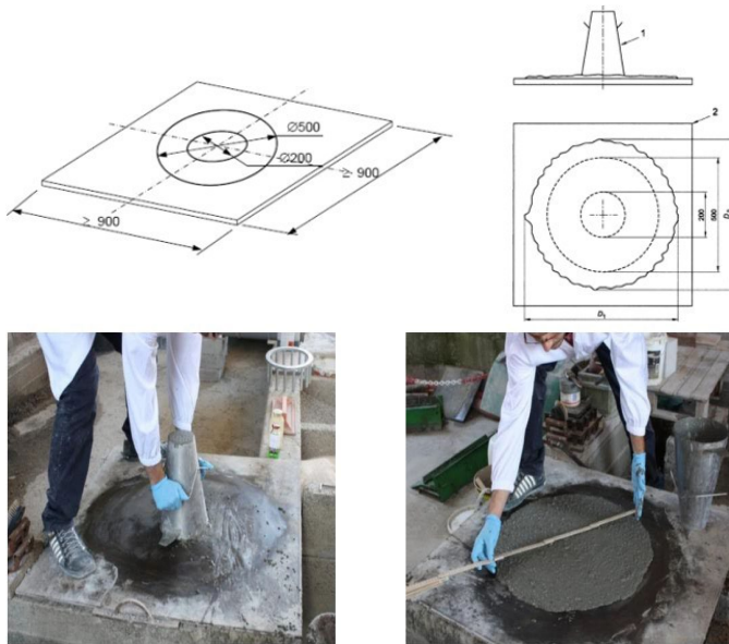
Fig. 1. Slump Flow test
