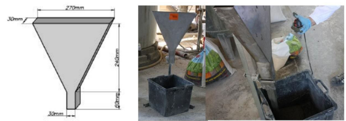
Fig. 2 V funnel test.
