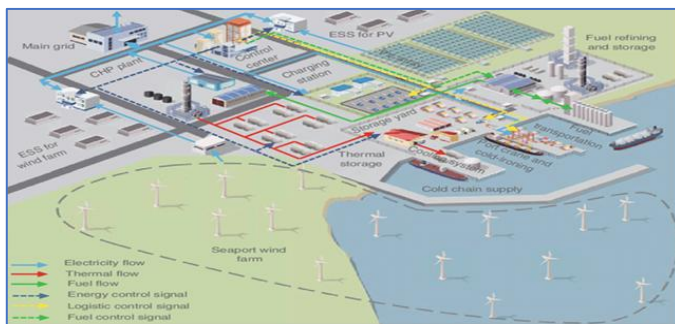
Fig. 8. Schematic of the Seaport Multi Energy Distribution. [49]
