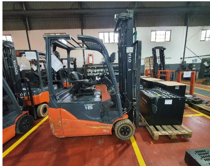
Fig. 3. Toyota Electric Counterbalance Model 8FBE16 (Own elaboration)
