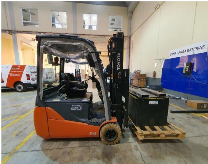
Fig. 2. Toyota Electric Counterbalance Model 8FBE20 (Own elaboration)
