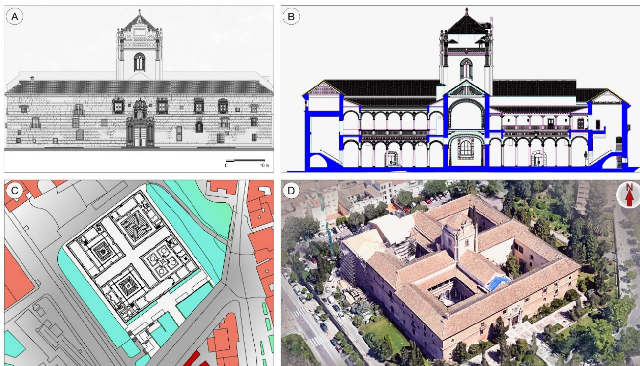
Fig. 1 Elevation plan (a), section plan (b), floor plan (c) and aerial view (d) of the Royal Hospital of Granada building
