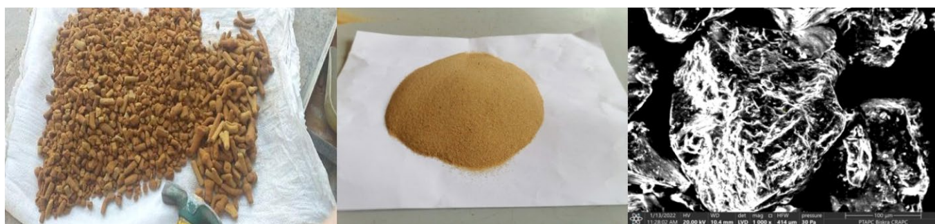
Fig. 1 Photography of WFS. Left: WFS cores; mid: WFS crushed; Right: Morphology of WFS particles (from SEM)
