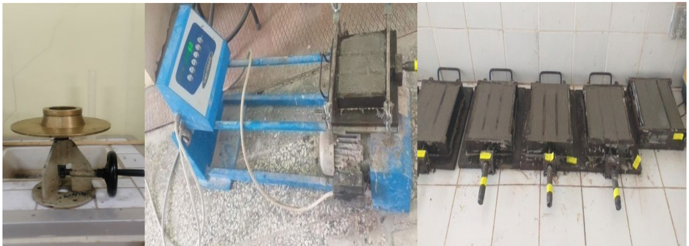
Fig.4. Manufacturing of specimens. Left: Flow table test; Mid: Jolting table; Right: Mortar specimen.
