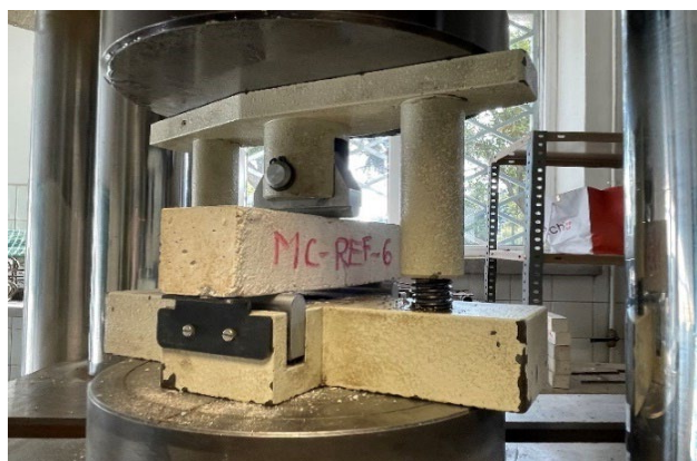
Fig. 6. 180-day flexural test. Source: Photograph by author
