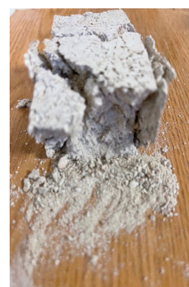
Fig. 7. 180-day compressive test. Source: Photograph by author
