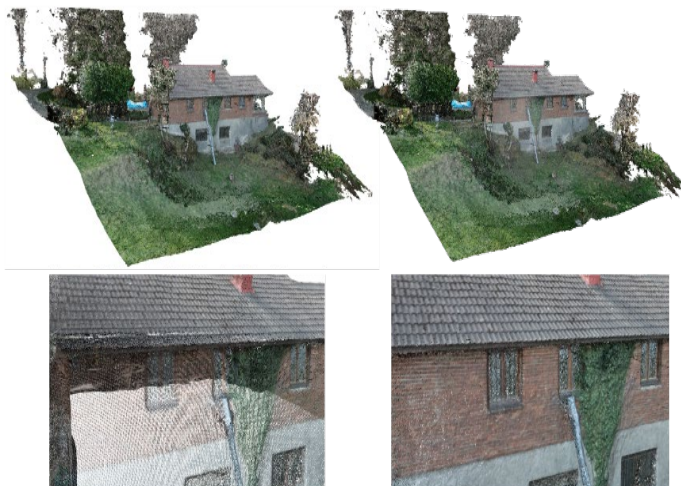
Fig. 5. Dense point cloud models: a) Medium quality b) High quality (Source: Own elaboration)..
