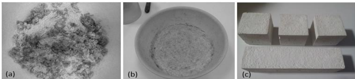
Fig. 1. Materials before kneading (a), consistency of the paste obtained (b), un-moulded specimens (c). Source: [27, Fig.3.11, 3.12, 3.14].
