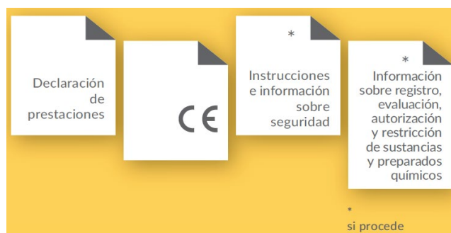
Fig. 3. Documentation to be handed over to the customer. Source: "CE marking of construction products step by step" published by the European Commission, p. 13).
