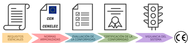
Fig. 1. Functioning of the CE marking system for construction products. Source: own elaboration.
