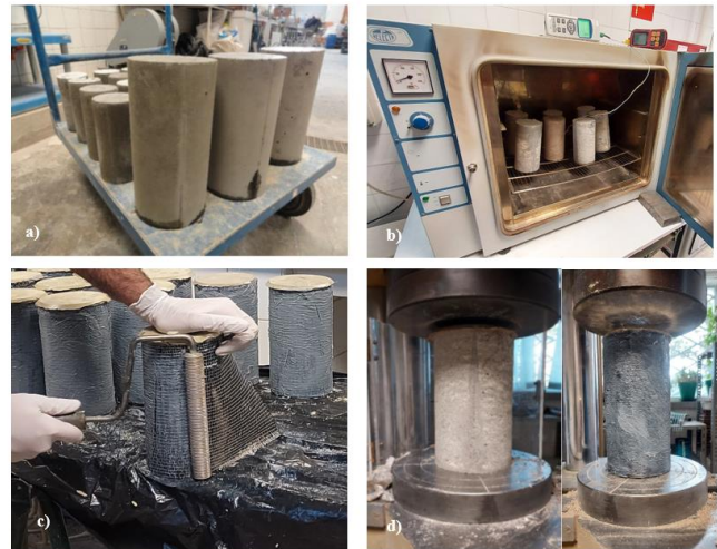
Fig. 1. Experimental process. a) Fabrication; b) Heating; c) CFRP reinforcement; d) Compression test.
