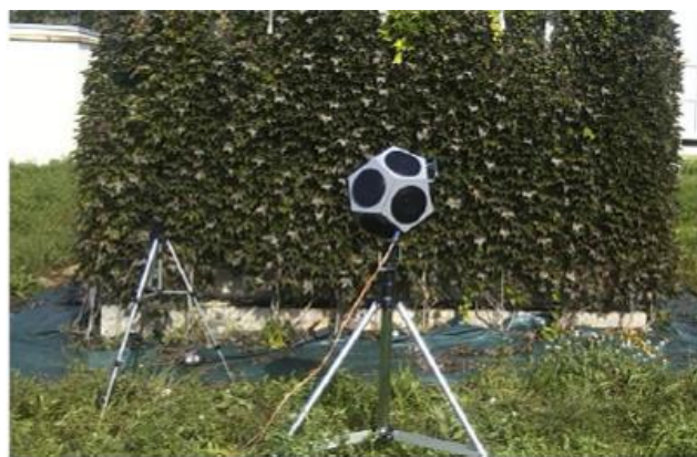
Fig. 11. Data collection for the evaluation of the acoustic insulation capacity of vertical greening systems for buildings (Azcorra et al., 2015; Pérez et al., 2016).
