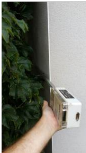
Fig. 10. Indirect measurement (ceptometer) of LAI in a Green facade and co-relation with the building facade wall exterior surface temperature (Pérez et al., 2017).
