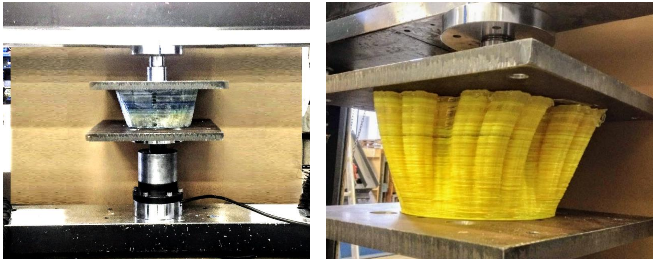
Fig. 29. Minimal deformation and improved strength in polyhedral cell and fractal shell tests.
