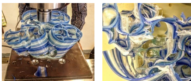
Fig. 27. Failure detail of token 1.
