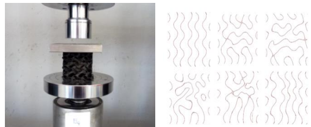
Fig. 10. Algorithmically differentiated token with toolpath contour every 10mm.
