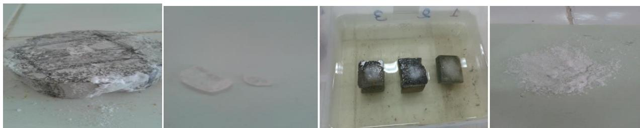
Fig. 19. Material formed on samples during sulphate attack.
