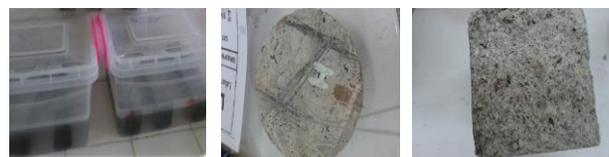
Fig. 5. Concrete and mortar samples for sulphate attack
