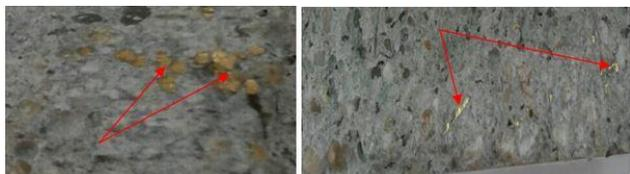
Fig. 9. Color of the fibers on the surface of the mortars.
