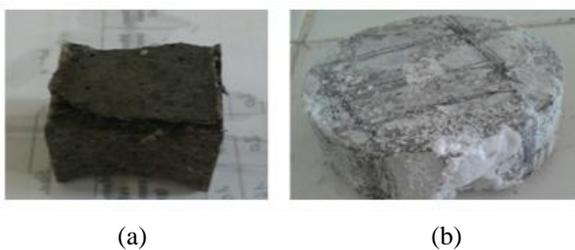
Fig. 13. Samples after sulphate attack. (a) Mortar. (b) Concrete.
