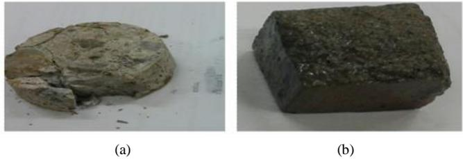
Fig. 22. Degraded state at 45 days of acid attack: (a) Mini-cylinders of concretes. (b) Cubes of mortars.
