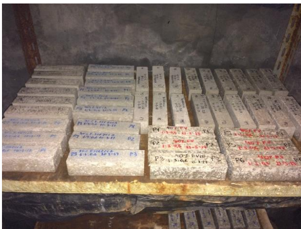
Fig 8. Cured specimens in a humid chamber.
