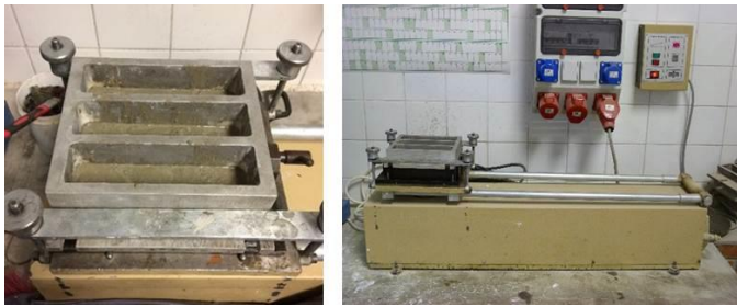
Fig. 7. Filling specimens on mechanical compactor.
