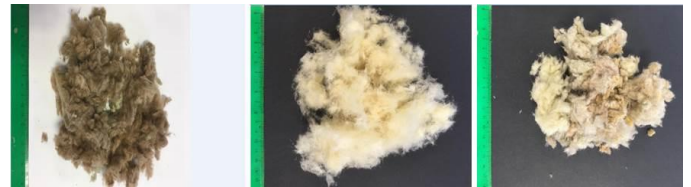
Fig.4. Material used in experiment, from the left: rock wool, fiber glass and mix both.
