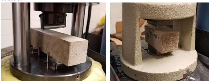
Fig 9. Test for flexural (left) and compressive (right) strength.
