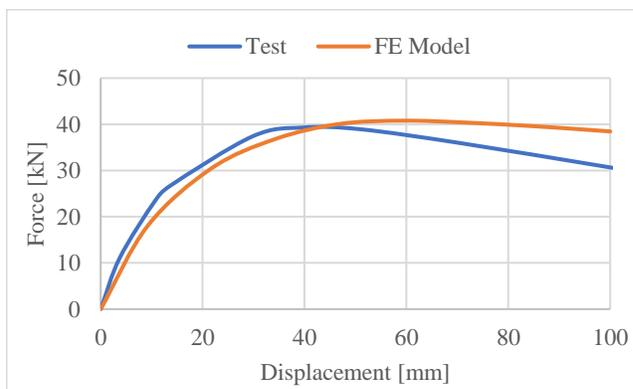
Fig. 6. Force-displacement curves obtained from the cyclic test and the numerical model.
