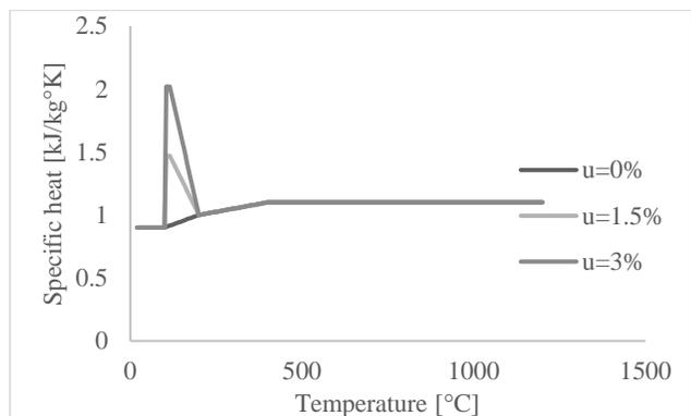
Fig. 2. Variation of specific heat as a function of temperature for moisture content 0%, 1.5% and 3% (CEN, 2004).
