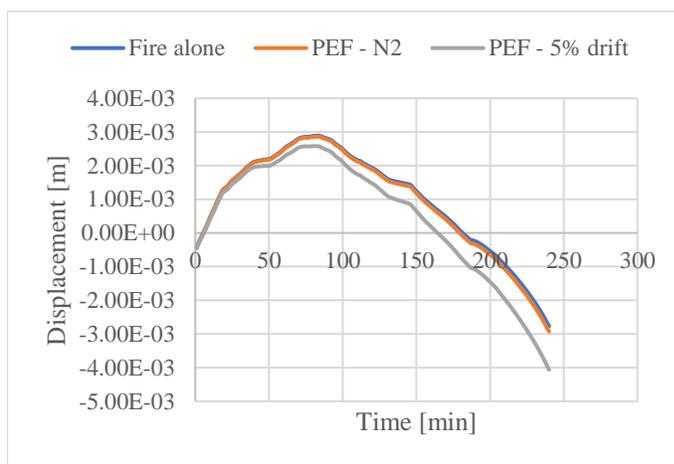
Fig. 11. Variation of the first-floor vertical displacement as function of time
