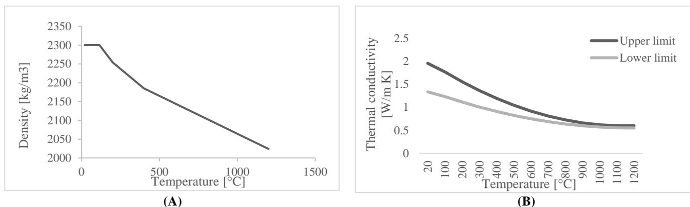
Fig. 1. (A) Variation of concrete density as a function of temperature, (B) Variation of thermal conductivity of concrete as a function of temperature (CEN, 2004)
