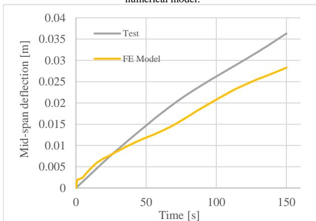
Fig. 7. Comparison of measured and predicted mid-span deflection.
