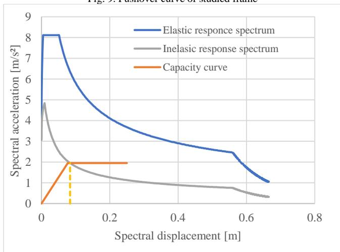
Fig. 10. Idealized capacity curve with response spectra
