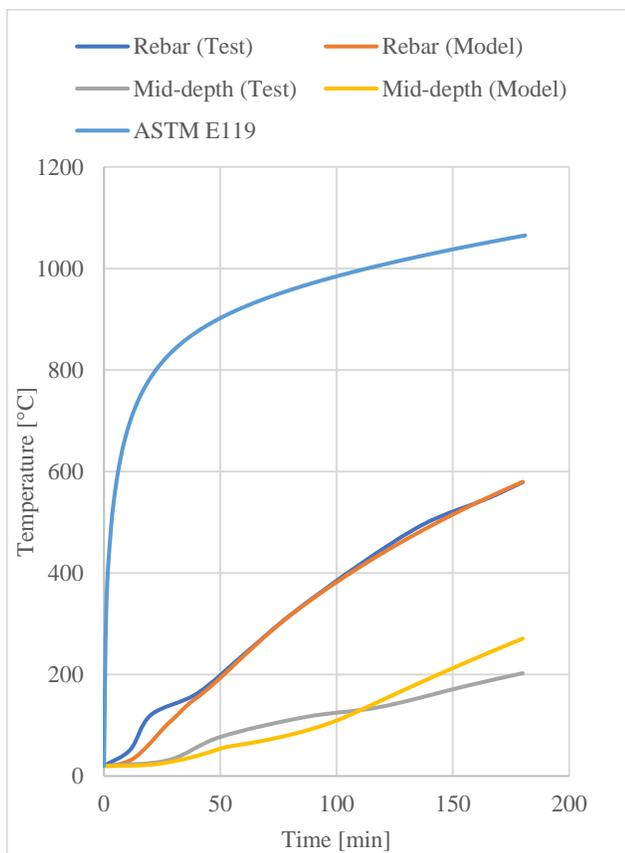
Fig. 5. Comparison of temperature evolution in the tested and calculated beam as a function of time
