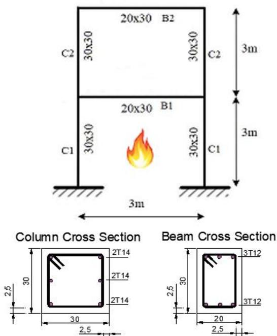
Fig. 8. Frame geometry.
