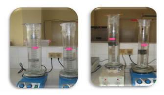
(a) (b) Fig. 4. Leaching device: a) On concrete disc; b) On cube of mortar.
