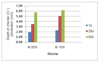
Fig. 31. Depth of penetration of Cl<sup>-</sup> ions.
